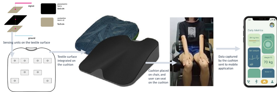
Figure 4. (a) Pressure sensors positioned for posture monitoring; (b) ergonomic cushion design with replaceable cover; (c) person using the cushion; and (d) application interface displaying real-time data and exercise guidance.
