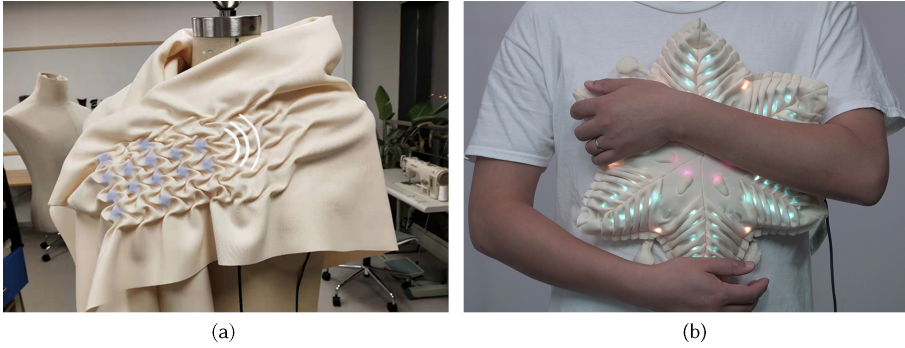
Fig. 8. (a) the smart shawl prototype for self-emotion regulation in daily life; (b) the iPillowPal prototype for remote emotional communication and interaction using affective gestures.
