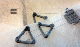
Figure 1: Examples of conductive yarns and 3D printed structures.
